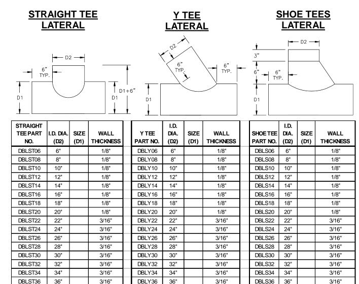
This table above is extrapolated in accordance with the ASTM D 3982-92 Standard Specifications for Contact-Molded Fiberglass Duct and Hoods (replaces NBS Voluntary Product Standard PS 15-69). Non standard sizes, flanges, straights, and bell ends priced on request.
